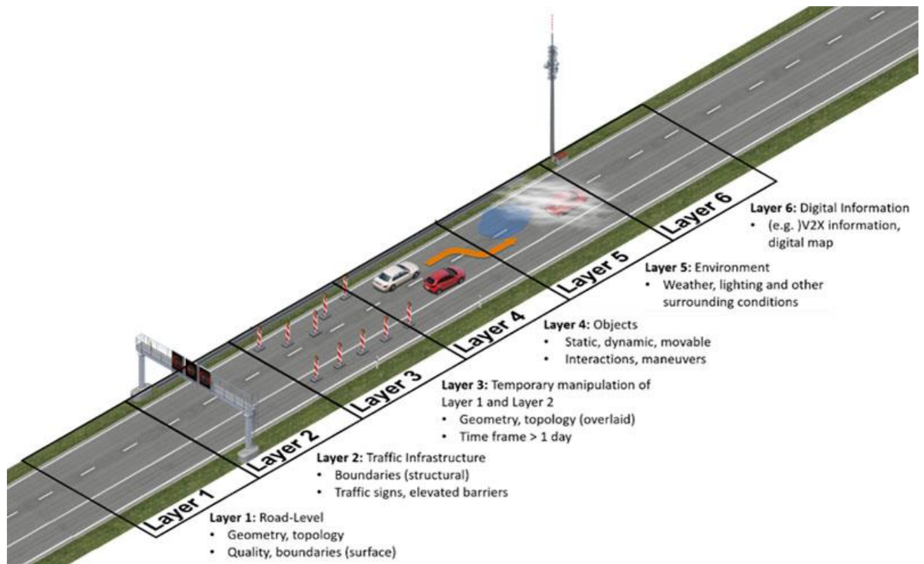
Figure 10: Scenario layers as defined in the PEGASUS method. Source: PEGASUS (2019)
